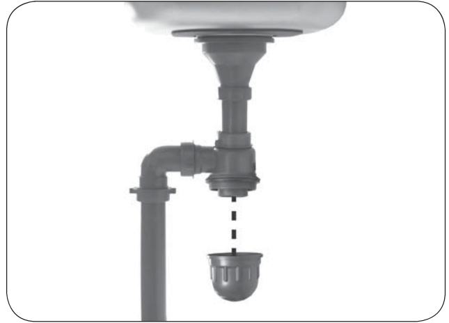
Fig. 4-1 Drain trap cleaning
