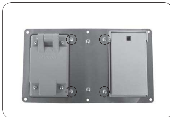
Fig. 36-3 Remove 4 small screws
