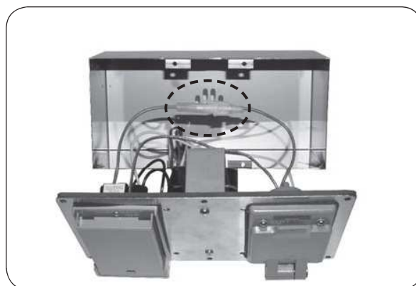
Fig. 36-4 Carefully open box and replace fuse (red wire)
