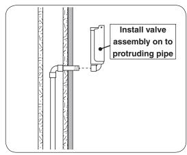
Fig. 2-1 Install valve assembly
