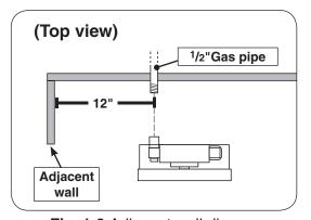
Fig. 1-3 Adjacent wall diagram
