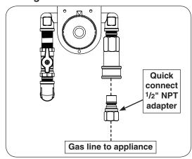
Fig. 2-3 Connect to gas line
