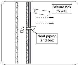
Fig. 2-2 Install stainless steel box
