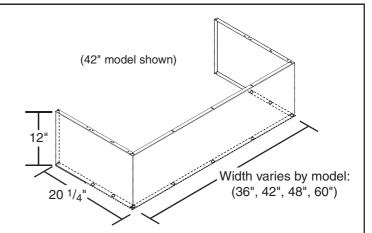
This Fire Magic Duct Cover is specifically designed for your Fire Magic Vent Hood. To install, read and follow <u>all</u> instructions in the owner's manual provided with your vent hood.
