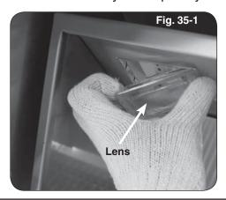
**5.** Wearing a pair of gloves, reach into the fixture, gently grab the bulb, and pull it straight out of the fixture so that the two pins at the base of the bulb come all the way out.
