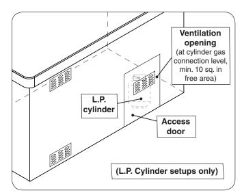
Fig. 9-2 Additional ventilation opening for L.P. cylinder
