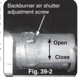
Too large an air shutter opening will allow too much air into the burner, which will cause the flames first to shorten and then to appear to lift up off the ports. For the bottom of the flames to move closer to the ports, close the air shutter more.
