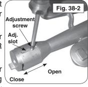
with a screwdriver, then sliding the air shutter backward or forward to open or close the air shutter opening (see Fig. 38-2).
