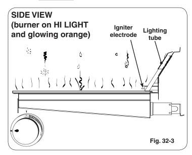
Drips and particles evaporate before hitting infrared burner when cooking at the maximum setting.
