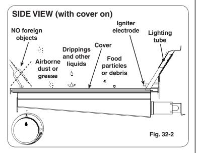
Burner ceramic must be protected with cover when burner is not in use.
