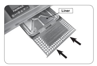
Fig. 22-3 Install drip tray
