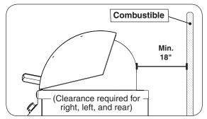
Fig. 11-3 Clearance 'C' Diagram
