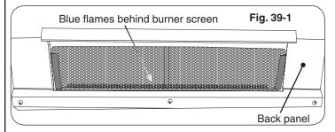
Flames from a properly adjusted backburner will appear as a horizontal line of even blue flames along the bottom of and behind the backburner grating. The grating itself will glow red after it heats up.
