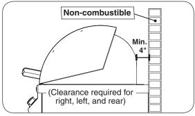
Fig. 11-1 Clearance 'A' Diagram
