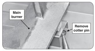
Fig. 41-2 Main burner removal
