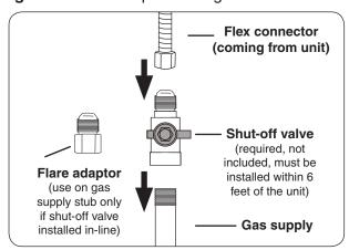
Fig. 20-3 Connecting to a gas line
