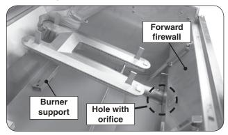
Fig. 41-3 Remove burners
