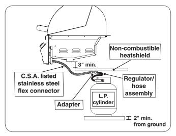
Fig. 9-1 L.P cylinder orientation
