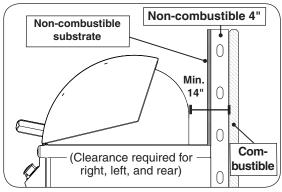
Fig. 11-2 Clearance 'B' Diagram
