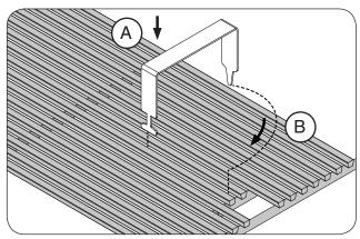
Fig. 22-1 Install cooking grids
