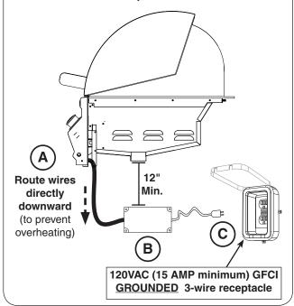
Fig. 23-1 Electrical installation
