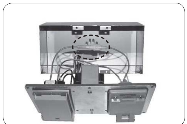
Fig. 32-4 Carefully open box and replace fuse (red wire)
